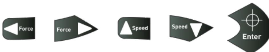
In order to set the correct starting point for plotting, in offline mode, move the cutter head and foil in such a way, that the laser point is located in the so-called start box in front of the bar code on the inserted medium. Now confirm the zero point by pressing the crosshair, which will cause the device to automatically switch to online mode.
