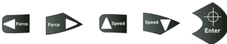
In the offline mode, the cutting head can be moved left and right by pressing the „Force“ arrow keys, as well as forwards or backwards by pressing the „Speed“ arrow keys. The corresponding X and Y coordinates are shown on the display.
