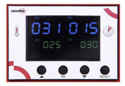
With a large digital controller, temperature (°C und °F) and pressing time can be adjusted. The green digits are showing the theoretical value, the white digits are showing the actual value. A counter (at the right bottom) counts the number of transfers that have already been made during the current session. The counter can be reset at any time.
